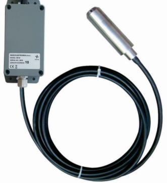
Levelwatch BLE-P is hydrostatic pressure wireless tank level monitor for smartphones. Sensor continuously measures the level and sends data to smartphone via Bluetooth. Data from sensor is monitored with the use of free LevelWatch application for IOS/Android smartphone. Drop-in sensor is suitable for clean liquids.
